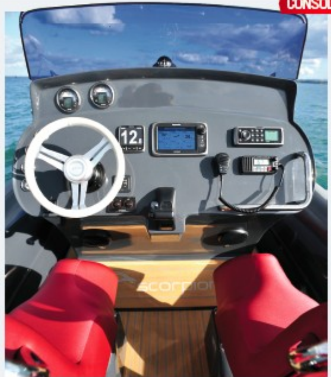
Caution here: leading edge of windscreen possible hazard.
